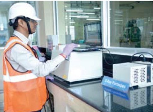
4. Surface Chrome (Passivation) Measurement (PORTASPEC)
