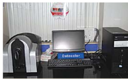
9. Machine Colour Match (Datacolor Spectrophotometer)
