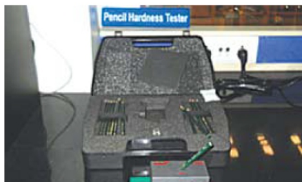
10. Paint Film Hardness (Pencil Hardness Tester)
