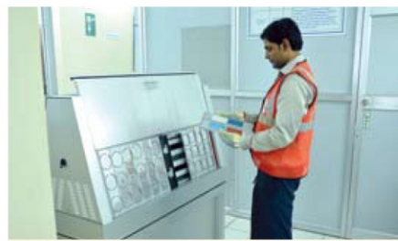
12. Colour Fading (Q-UV Tester)
