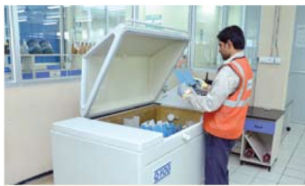
11. Corrosion Resistance (Q-Fog Salt Spray Tester)
