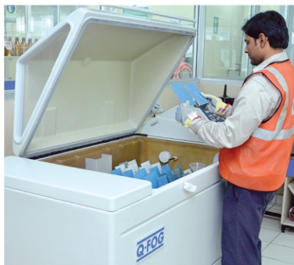
Salt Spray Corrosion Resistance Testing
